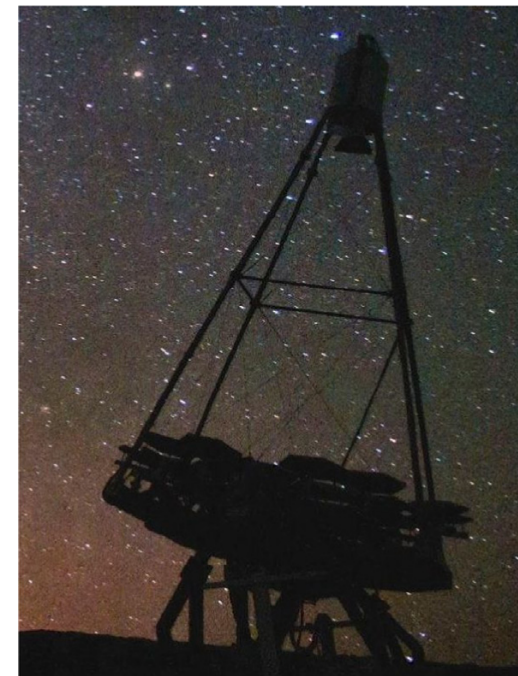
Fig. 1. Photo of the First G-APD Cherenkov Telescope during data taking (P.Vogler). The mirror has an area of \approx 9.5 \text{ m}^2 , and the camera consists of 1440 G-APD pixels with a total field of view of about 4.5^\circ .
