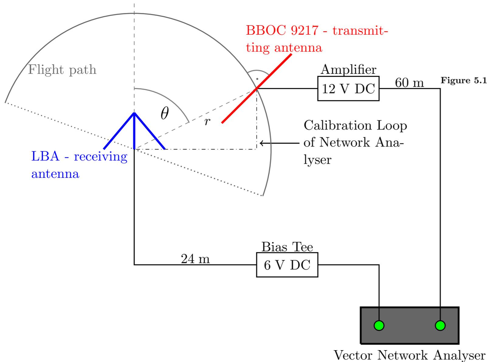
**Figure 5.3:** Set-up to measure the horizontal gain. The grey half circle denotes the path of the transmitting antenna. The angle  $\theta$  highlights the zenith angle of the transmitting antenna with respect to the LBA. The black dashed-dotted line indicates the cable connection between the LBA and the amplifier used for the calibration of the network analyser. Modified figure from [41].
