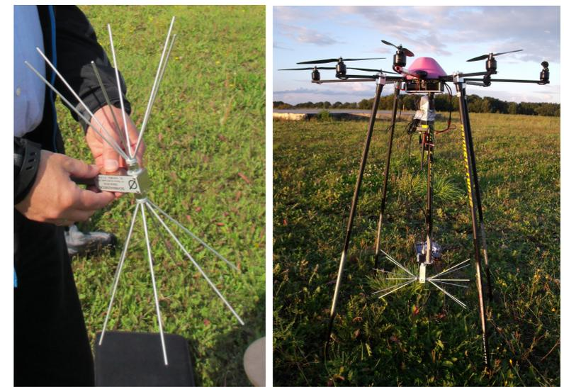
**Figure 5.1:** *Left:* Biconical antenna used for the calibration measurements. *Right:* Octocopter with the transmitting antenna mounted below.
