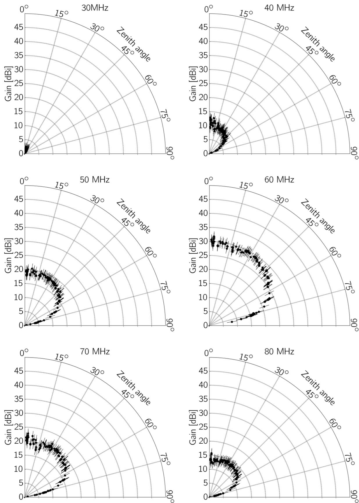
**Figure 5.12:** Measurements of the horizontal gain of the outer LBA as a function of zenith angle for different frequencies. The error bars indicate the systematic uncertainty caused by the frequency analyser and the biconical antenna. The statistical errors are small compared to the systematic ones. The error bars of the zenith angle are smaller than the marker size.
