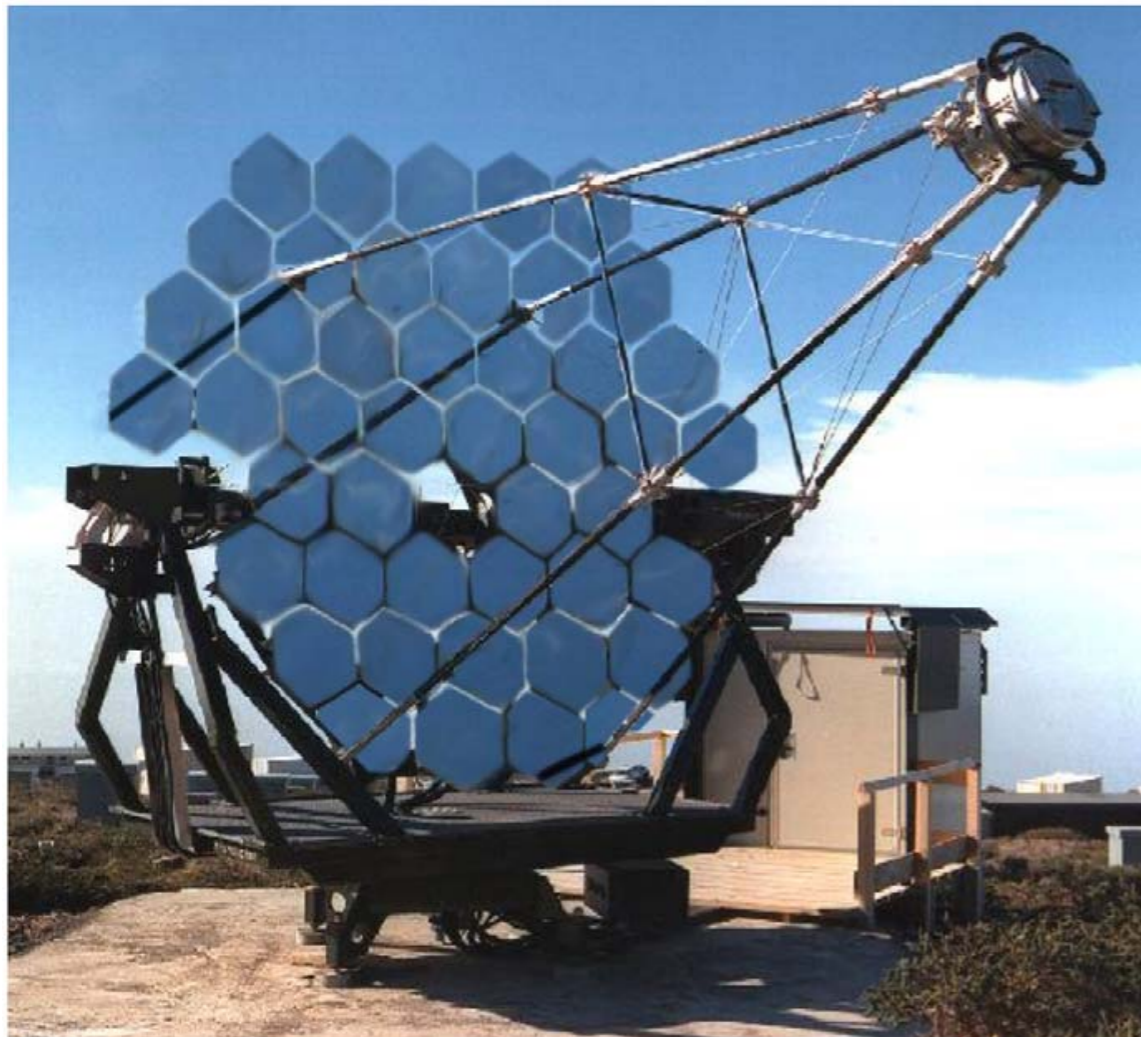
Fig. 1. A photomontage of the refurbished HEGRA CT3 telescope with \sim 13 \text{ m}^2 mirror area (La Palma, Canary Islands, Spain).
