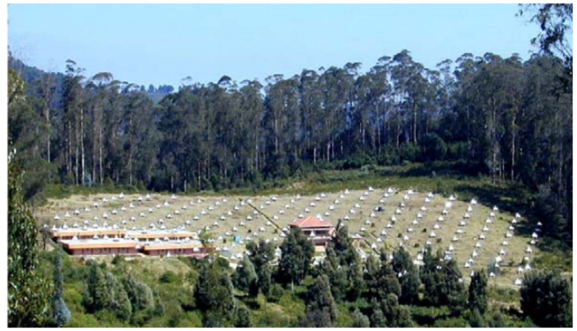
Fig. 2. A view of the GRAPES-3 array showing electron detectors and the central control room. Four halls housing the muon detectors are seen on the left. The detectors lined up from the top-right to the bottom-left in the picture, are along the East to West direction.
