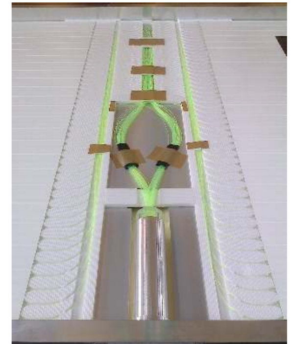
Figure 3: Routers for guiding and protecting fibers on the side ( left ) and in the center ( right ).
