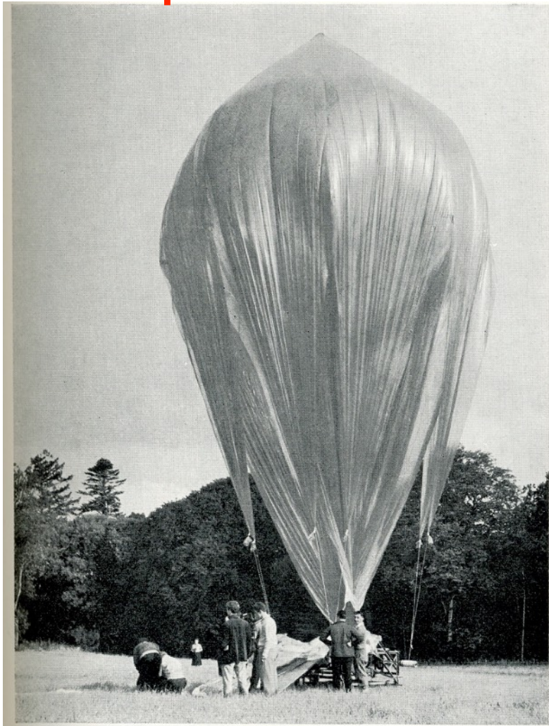
Fig. 1. Inflation of balloon of polyethylene just after dawn. The balloon has a total length of about 120 ft. and most of the fabric is on the ground. Such a balloon can in favourable conditions give level flight at about 90,000 ft. for many hours with a load of 40 kg.
