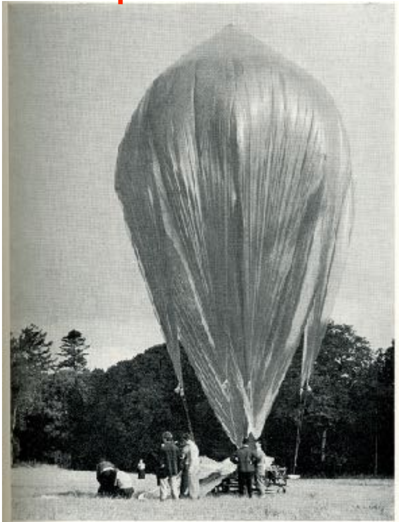
Fig. 1. Inflation of balloon of polyethylene just after dawn. The balloon has a total length of about 120 ft. and most of the fabric is on the ground. Such a balloon can in favorable conditions give level flight at about 90,000 ft. for many hours with a load of 40 kg.
