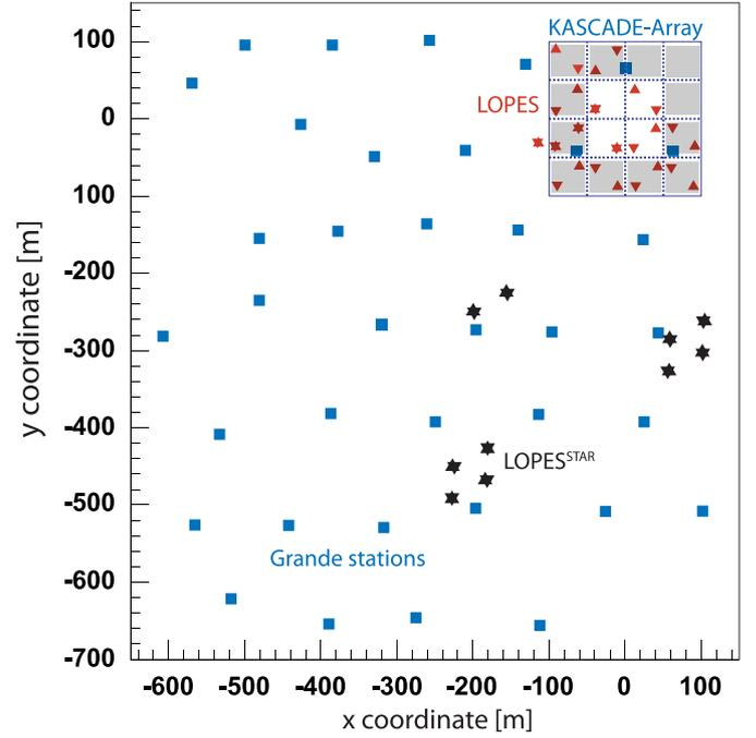
**Fig. 1.** The KASCADE-Grande Facility. Small squares represent the Grande stations. The KASCADE array is seen at the upper right hand of the figure. KASCADE detectors are arranged in 16 clusters. The outer 12 clusters contain muon detectors. LOPES antennas are displayed by triangles, i.e. a star signs a dual-polarized antenna with two channels.
