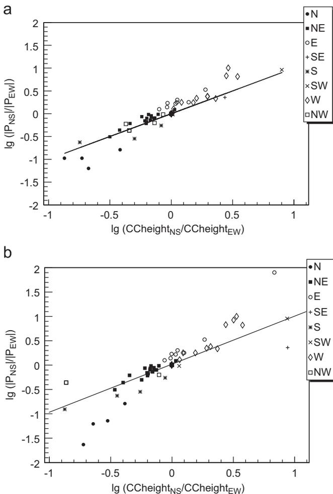
**Fig. 3.**  $|\vec{v} \times \vec{B}|_{NS}/|\vec{v} \times \vec{B}|_{EW}$  vs. the ratio of the pulse heights for the NS and EW polarizations, in the case with pedestal (a), and without pedestal (b). The different markers denote air shower arrival directions.
