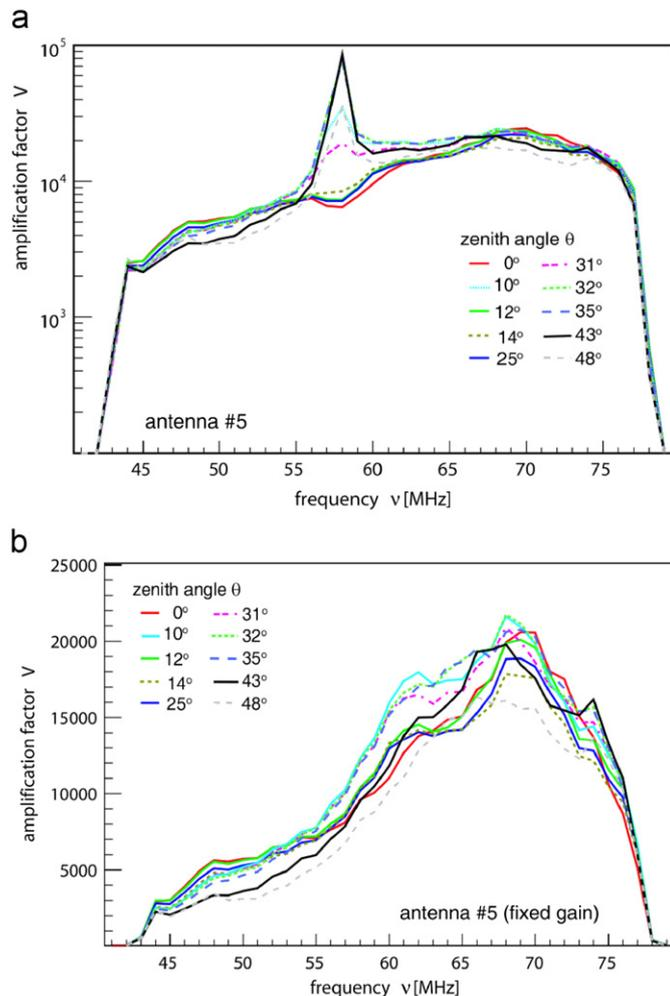
**Fig. 1.** Amplification factor distribution for one antenna for different zenith angles, with the metal pedestal included in the simulation (a), and without metal pedestal included in which case  $G_t$  is fixed to 4.0 [5].
