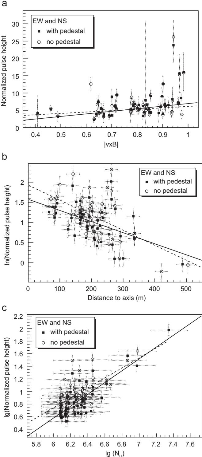
**Fig. 2.** Dependence of pulse height on polarization vector modulus,  $P = |\vec{v} \times \vec{B}| = \sqrt{(P_{EW}^2 + P_{NS}^2)}$  (a), on distance from antennas to shower axis (b) and dependence of  $\log_{10}$  of pulse height on  $\log$  of muon number.
