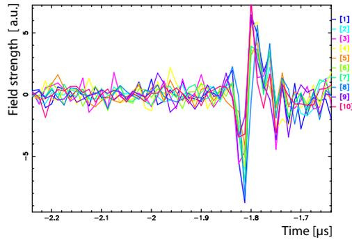
Figure 2: Raw signals of the individual antennas for one event example. The signals at this stage are prepared for the beam-forming based on shower observables reconstructed by KASCADE-Grande.
