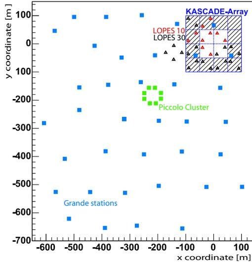
Figure 1: Sketch of the KASCADE-Grande – LOPES experiment: The 16 clusters (12 with muon counters) of the KASCADE field array, the distribution of the 37 stations of the Grande array, and the small Piccolo cluster for fast trigger purposes are shown. The location of the 30 LOPES radio antennas is also displayed.
