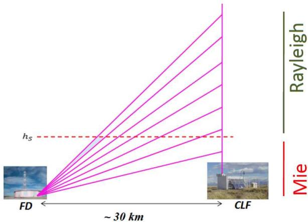
Figure 1: Schematic representation of the propagation of laser photons from the CLF to the FD site. In this model, there is an aerosol band in the area below the  $h_S$  horizontal line. Rayleigh and Mie scattering dominated regions are, respectively, above and below the scale height parameter,  $h_S$ .
