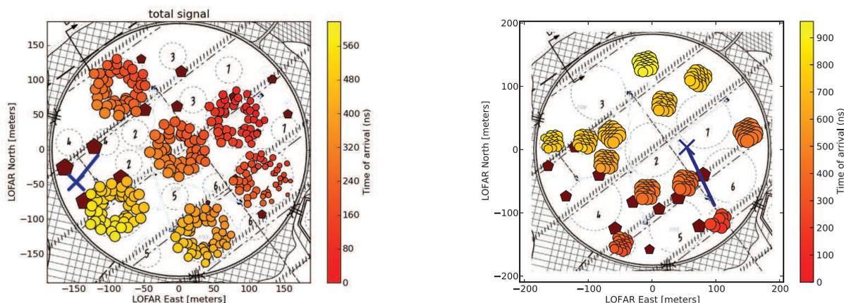
**Figure 5:** Footprints of two air showers measured by LOFAR with the low-band antennas (30 – 80 MHz, *left*) and the high-band antennas (110 – 240 MHz, *right*). Circles represent the radio antennas, pentagons the scintillator detectors. The symbol size is proportional to the measured signal strength. The color denotes the arrival time.
