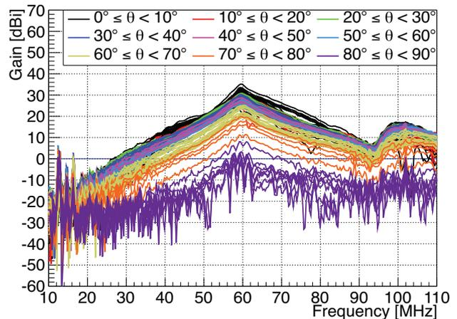
**Figure 2:** Measured antenna gain as a function of frequency.
