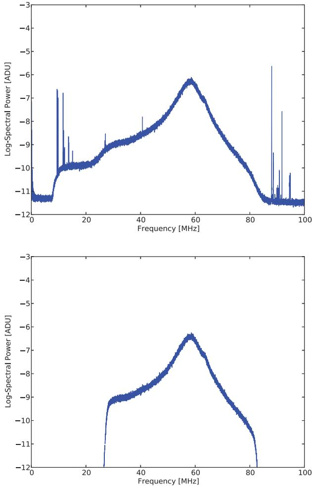
**Figure 3:** The average spectrum of a typical LBA event (*top*) and cleaned from RFI and clipped to 30 – 80 MHz (*bottom*).
