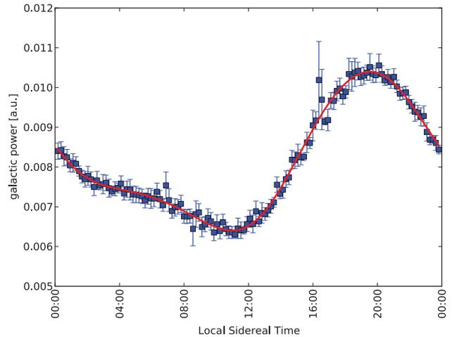
**Figure 4:** The integrated spectral power, normalized to the bandwidth, after RFI cleaning as a function of local sidereal time for the north-east south-west polarization direction.
